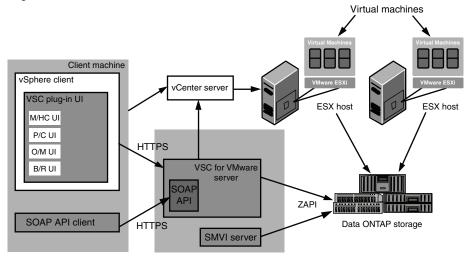
The following diagram provides a high-level overview of the VSC for VMware vSphere architecture:
